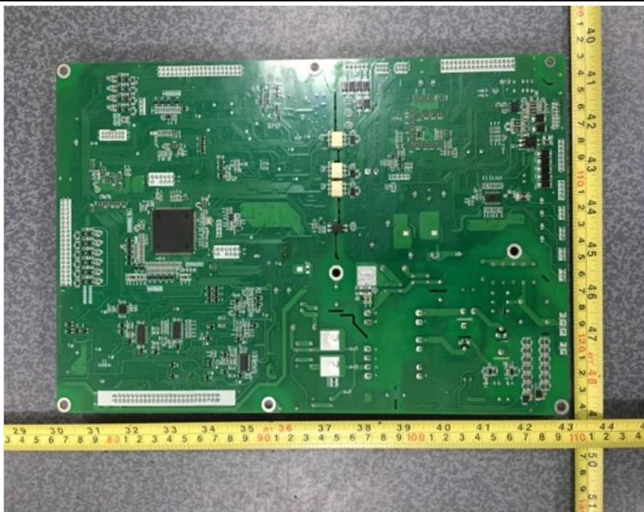
Back side of Control board
