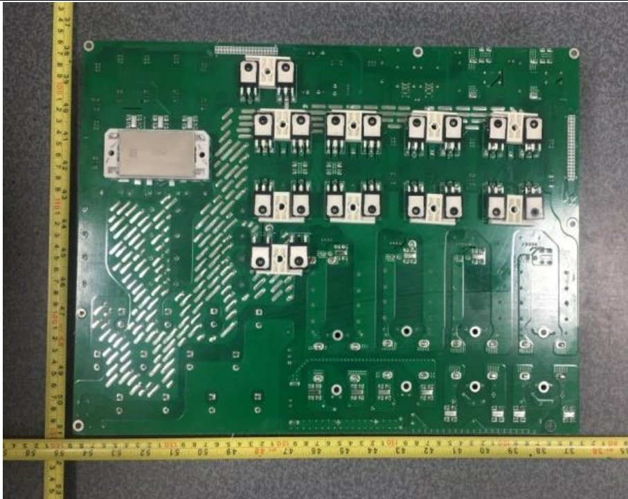
Back side of Power board
